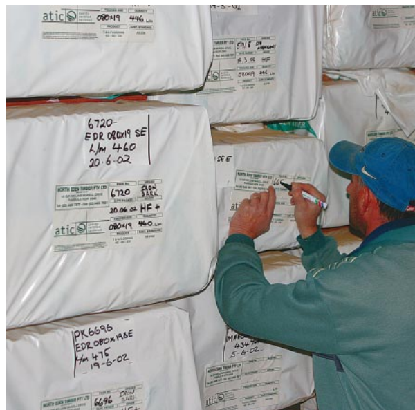
Correctly packaged and labelled with the grade, compliance standards and producer's name.
